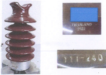
Figure 1 Line-Post type porcelain insulator class 57-2, Lot No. 111-240, under test.
