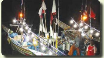
To lower greenhouse gas emissions resulting from power-generating engine combustion, PEA investigated the feasibility of employing LEDs in fishing vessels that relied on lights to lure marine lives. To this end, it surveyed prototype fishing boats in Chon Buri, collected data on energy and productivity of these boats before and after LED conversion, and analyzed technical, economic, community, and environmental aspects of outcomes.
